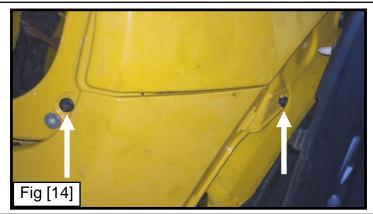
Step 9. Disconnect the bumper from the vehicle starting at the driver side. Use a flathead tool to release tabs located at the tail light assembly area. Continue removing the bumper until you have reached the passenger side. See Figure [15]. WARNING: Do not completely remove the bumper to avoid wire damage!
