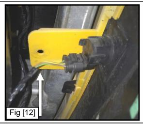
**Step 7.** Gently pull on fender flares starting at the rearward end, unsnapping as you go. Once pulled back you will notice a backup sensor attached. Gently disconnect the sensor harness. Repeat on opposite side of vehicle. See Figure [13].
